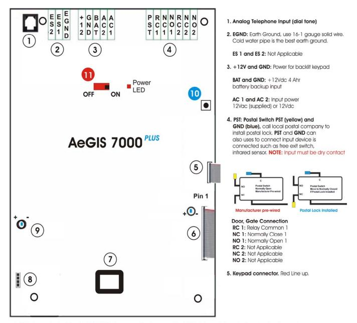
6. LCD Connector Red Line Up. WARNING: If you need to disconnect the LCD's ribbon cable, note down the direction and pins configuration. Connect the LCD's ribbon cable incorrectly, may damage the LCD or board. The RED LINE on the ribbon cable must be connected to pin 1.
